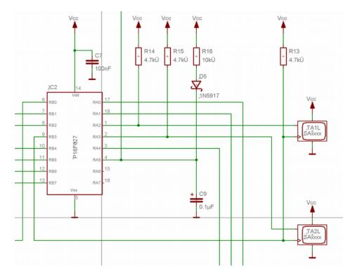
The SAxxxx keys are directly connected to the PIC16F627 controller. In this schematic we just see the clock and data lines of the SAxxxx switches. The contact matrix is not shown since it is not relevant for the communication.
