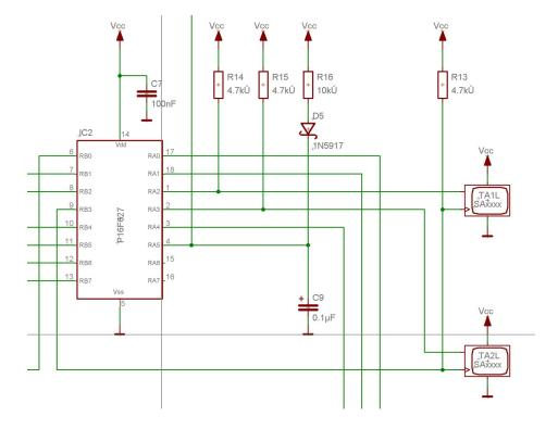
The Sx keys are directly connected to the PIC16F627 controller. In this schematic we just see the clock and data lines of the Sx switches. The contact matrix is not shown since it is not relevant for the communication.
