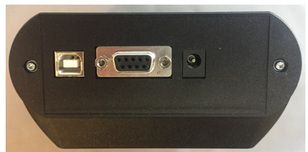
Fig. 1: CP0304 power connector (right), RS232 DB9 female connector (center) and USB Type B connector (left)
